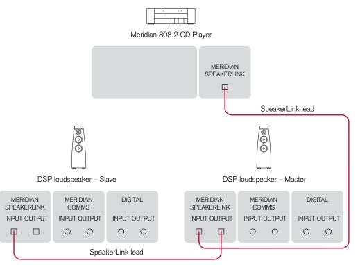
The 808.2/808.2i can be connected directly to Meridian DSP loudspeakers to create a complete compact stereo system, with volume and other preamplifier controls provided by the loudspeakers via the MSR+ or the front panel. The 808.2i provides additional analogue and digital inputs allowing you to use it to control the other sources in your system.
