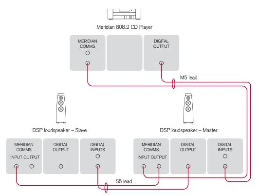
If your DSP loudspeakers do not provide Meridian SpeakerLink connections you can connect to them using the Digital and Meridian Comms connections.
